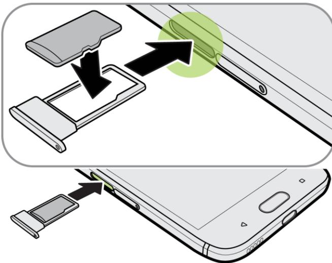
4. To reinsert the microSD card tray, center it first in the slot, and then slide it all the way in.
