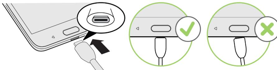
3. Plug the other end of the USB cable into the AC adapter.
