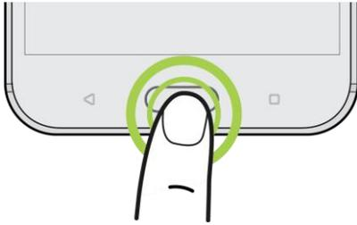
5. Repeatedly touch the scanner until the fingerprint has been successfully recorded. You'll get the best results if you hold your finger in the same direction when touching the scanner.
