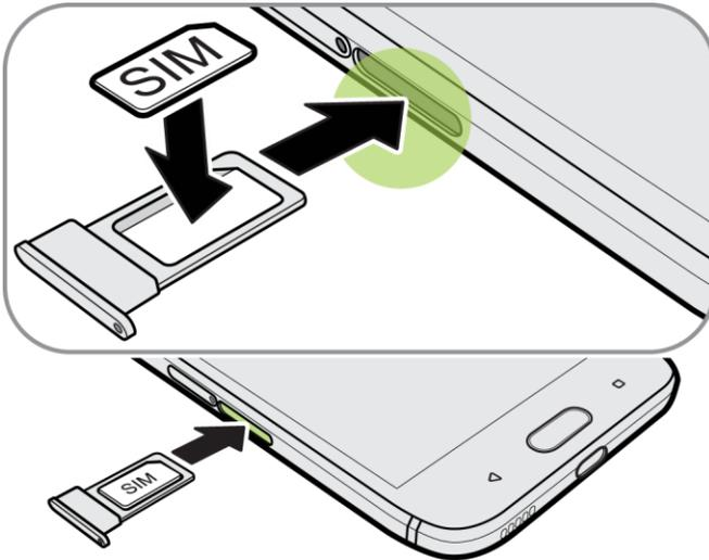
5. To reinsert the nano SIM card tray, center it first in the slot, and then slide it all the way in.
