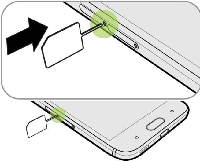
3. Pull the microSD card tray out, and place the SD card—contacts facing down—into the tray.
